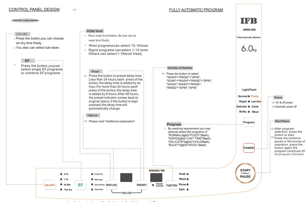
! In order to protect controller, the interval of switching on and off power should be more than 30 seconds.
